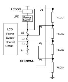
The internal resistors of LCD bias can be selected by software in SH67P54/P53. When large LCD panel is used, user can set the value of \$07 to increase the bias current for better LCD performance. But it will cost more power, User can also use external parallel connection resistances for complex bias current.
